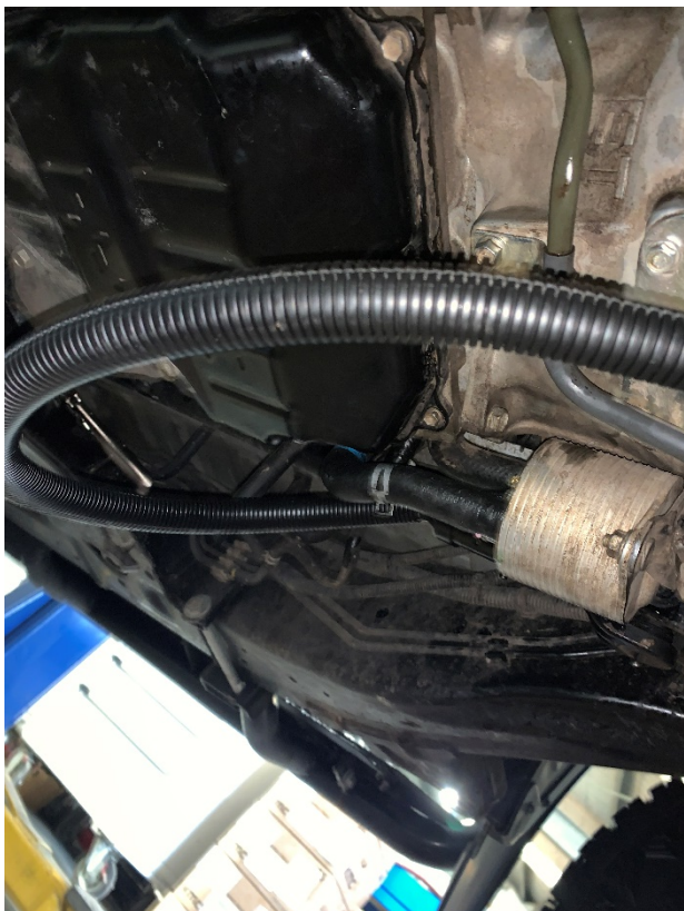
Step 6: You will then install the supplied hose onto the gearbox hose barb as shown.
