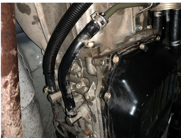
Step 6: You will then install the supplied hose onto the gearbox hose barb as shown.
