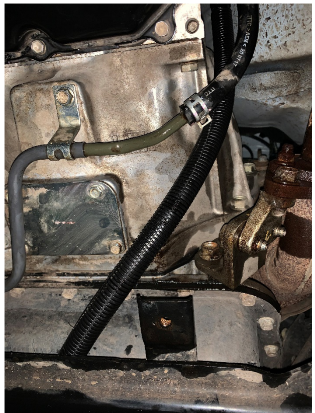
Step 7: Next you will run the hose as shown to protect them from being damaged and use the supplied zip ties to secure them to the car.
