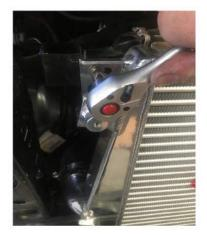
47. Click on the factory sensor plug on the bottom passenger side outlet.
