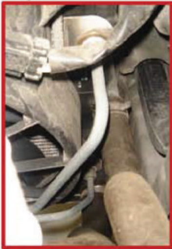
Fig 7: The Transmission Pipes
