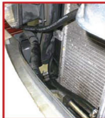
Fig 10: The Lower Transmission Cooler Hose
