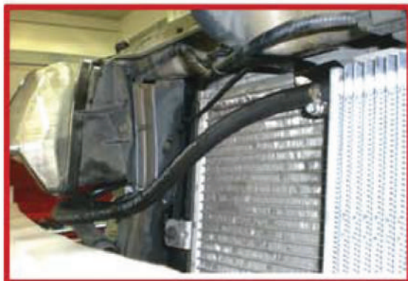
Fig 9: The Upper Transmission Cooler Hose
