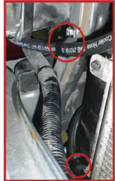
Fig 11: Secure Hose with Cable Clamps
