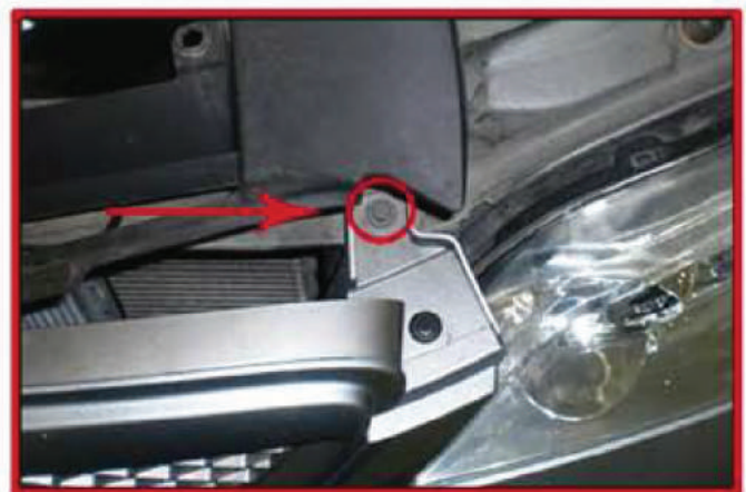
Fig 2: Lift Shroud to Access 2 Bolts
