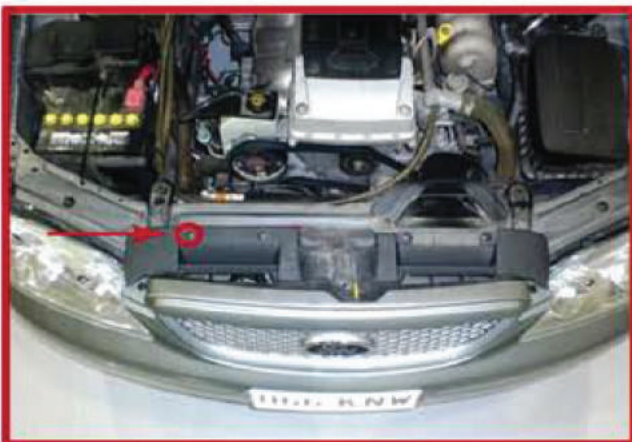
Fig 1: Remove 4 Scrivets from Shroud
